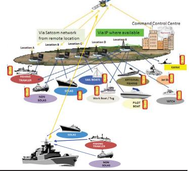
Patroling Navy or Coast guard Ships with vmsRECEIVER relays "out of coverage" area vessels to control station via SATCOM
