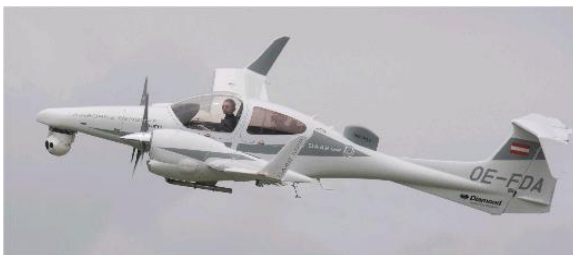
A DA42 MPP with SCOTTY Satcom antenna (top)
